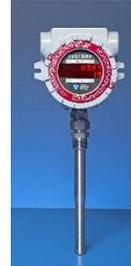
Model # 62-9 insertion probe with integral electronics (Model # 9500PI) with on-board menu system to allow for user initiated line size changes. The customer has cooling water line sizes ranging from 2" up to 24" and flow ranges up to 9000 GPM.
