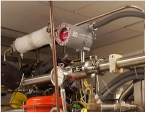
Thermal Instrument Company (TIC) manufactures a mass flow meter that can accurately and dependably measure the DI water solution used in CIP
